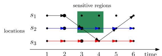
Fig. 3. We show two events, i.e.,  $\text{PRESENCE}(\mathcal{S}, \mathcal{T})$  and  $\text{PATTERN}(\mathcal{S}, \mathcal{T})$ . If the user's ground truth trajectory is the black one, only  $\text{PRESENCE}(\mathcal{S}, \mathcal{T})$  is true; if the user's trajectory is the blue one, both events are true; if the user's trajectory is the red one, both events are false.
