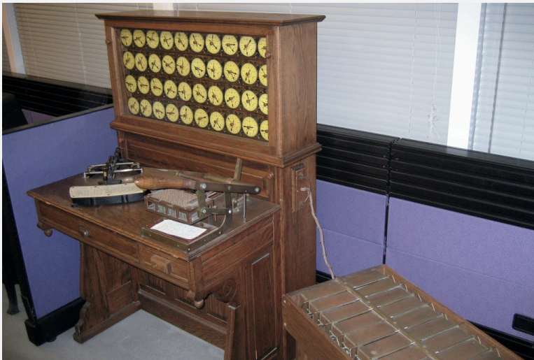
Hollerith tabulating machine and sorter
