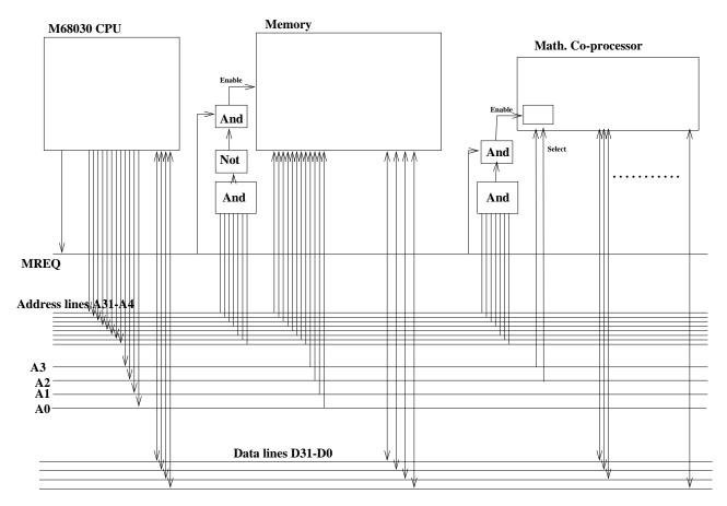
The memory will only enables if its **Enable** signal is equal to ONE.
