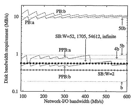
Figure 6: Disk bandwidth requirement (MBytes/sec).
