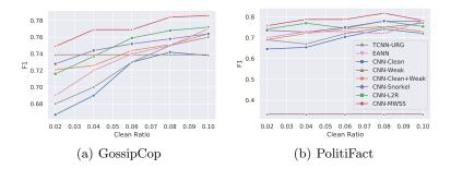
Fig. 4: F1 score with varying clean data ratio from 0.02 to 0.1 with CNN-MWSS. The trend is the similar with RoBERTa encoder (best visualized in color).
