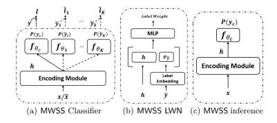
Fig. 2: The proposed framework MWSS for learning with multiple weak supervision from social media data. (a) Classifier: Jointly modeling clean labels and weak labels from multiple sources; (b) LWN: Learning the label weight based on the concatenation of instance representation and weak label embedding vector. (c) During inference, MWSS uses the learned encoding module and classification MLP  $f_{w_c}$  to predict labels for (unseen) instances in the test data.
